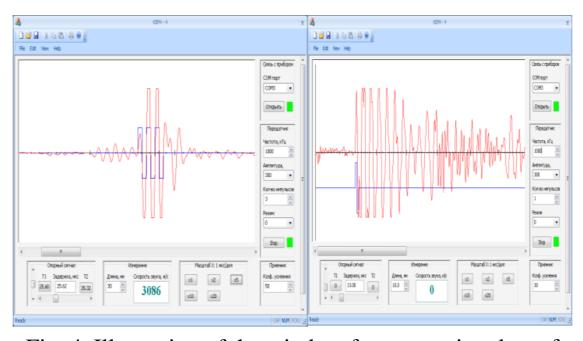
Fig. 4. Illustration of the window for processing data of elastic waves velocity  $V_{\parallel}$  measurements of computer device KERN-4
