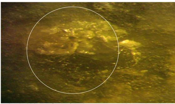
Fig. 2. SiO<sub>2</sub> surface after the nanosecond laser irradiation by the ruby laser with the intensity of I  $\approx$  300 Mw/cm<sup>2</sup> with the dose D = 4xI the duration of the ruby laser pulse  $\tau \approx 20$ ns with the wavelength  $\lambda = 694$  nm. The circle indicates the area of the laser irradiation (x56)
