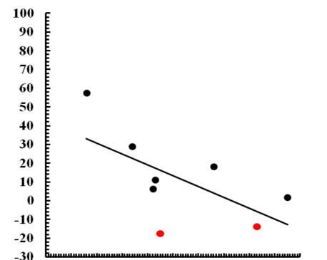
0 1 2 3 4 5 6 7 8 9 10 Km, % Fig. 6. Correlation dependence of the internal friction defect  $\Delta Q^{-1}/Q^{-1}$  in SiO<sub>2</sub> from the open porosity coefficient  $K_{PO} = V_{PO}/V$
