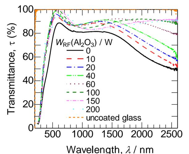
Effect of RF power of Al<sub>2</sub>O<sub>3</sub> target on transmittance of ITO50:Al<sub>2</sub>O<sub>3</sub> (PHS) thin films
