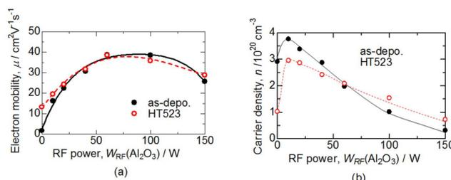
The electron mobility (a) and the carrier density (b) of the as-deposited and HT523 ITO50:Al<sub>2</sub>O<sub>3</sub> (PHS) thin films deposited at  $Q(\text{Ar})/Q(\text{O}_2) = 50$  sccm/0.1 sccm depending on RF power of Al<sub>2</sub>O<sub>3</sub> target
