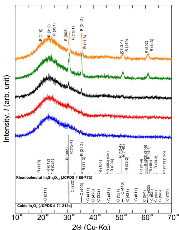
XRD results for as-deposited and heat-treated at 523-823 K ITO50:Al<sub>2</sub>O<sub>3</sub> (PHS) thin films
