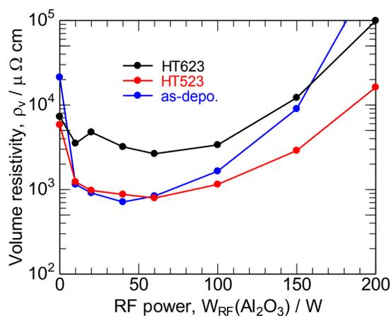
Effect of RF power of Al<sub>2</sub>O<sub>3</sub> target and heat treatment temperature on volume resistivity of the ITO50:Al<sub>2</sub>O<sub>3</sub> (PHS) thin films
