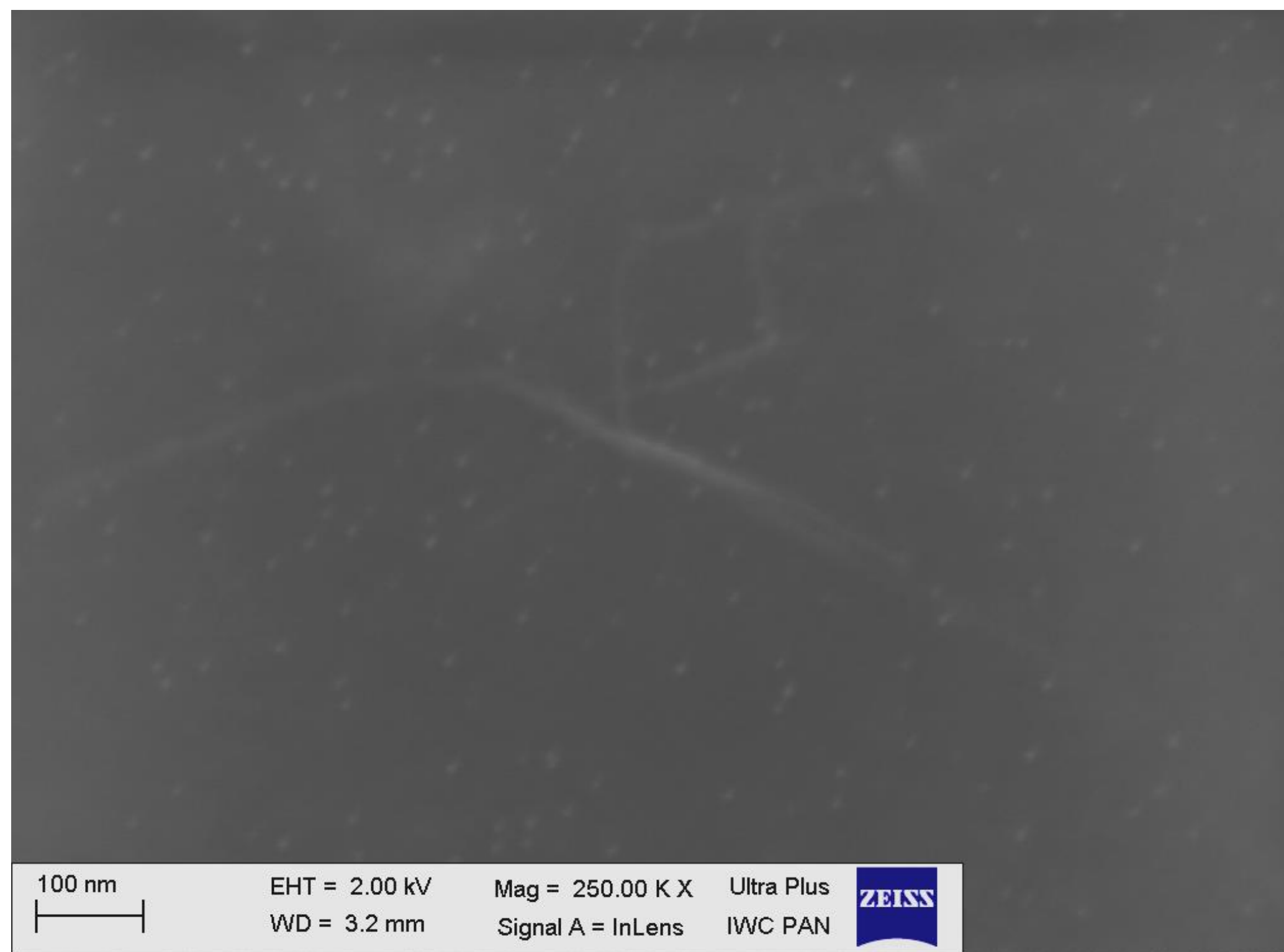
SEM image of a conductive path formed by several individual single-walled nanotubes inside PEDOT:PSS / 12 wt. % SWCNTs composite
