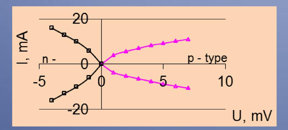
U-I characteristics of Si "X"- type joints: triangles p-type of conductance; squares – n-type of conductance
