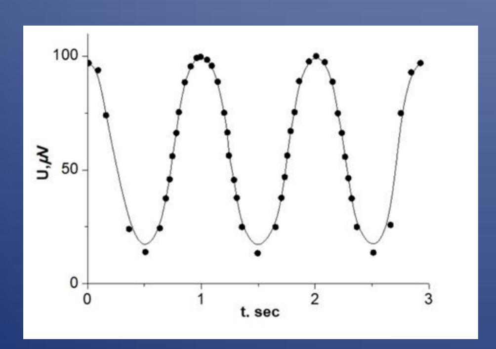
The measurement of U-I characteristics of Si nanowire joint were unexpected. When the current through the nanowire exceeds 10 µA the periodic oscillations of voltage arises. The period of oscillations is about 1 sec.
