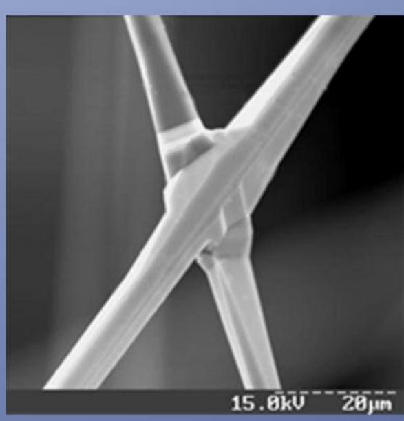
Si wire joints were obtained by crystallization from the gas phase through the liquid phase due to VLS mechanism. The wire diameter was about 50-100 nm.
