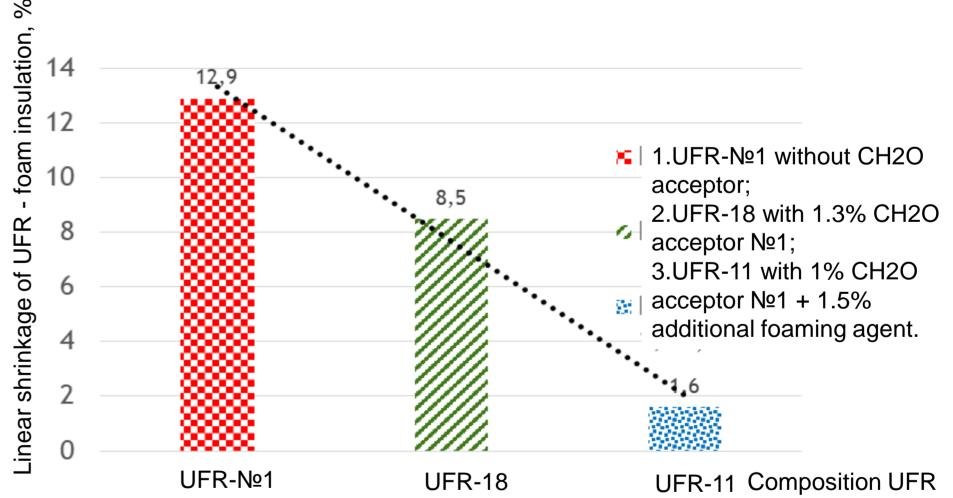
Fig. 2. Dependence of linear shrinkage of industrial foam insulation after production and drying 48 hours, (1-foam insulation without additives KFP-1; 2-foam insulation with the addition of formaldehyde acceptor KFP-18; 3-foam insulation with foamers and acceptor **KFP-11.**
