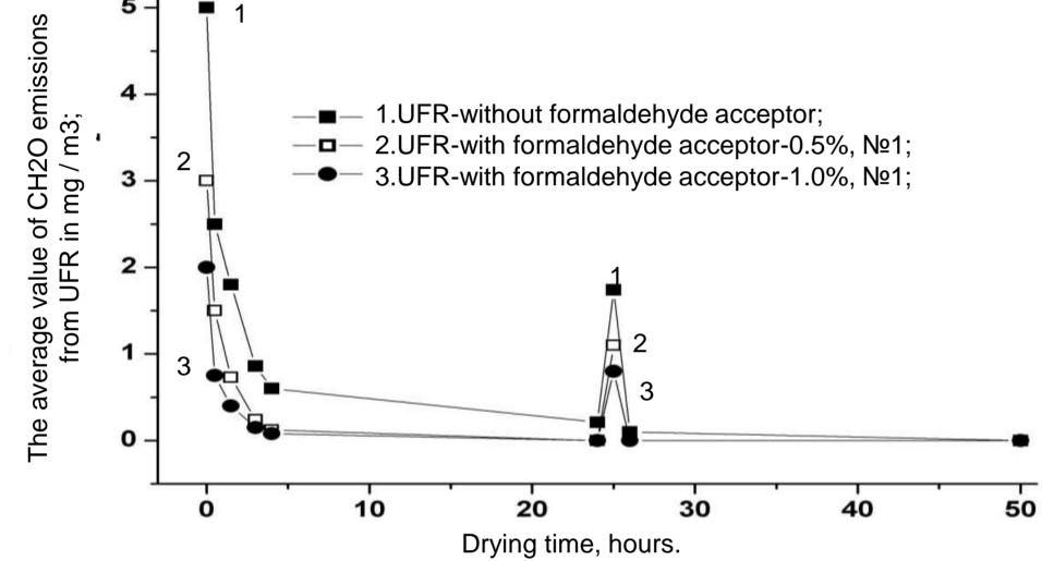
and chemical foaming agents. This led to a 2-3-fold reduction in the emission and concentration of free formaldehyde from urea-formaldehyde foam and a reduction in its volume shrinkage, and a decrease in water and moisture absorption of UFR. New chemical formaldehyde acceptors have been proposed that can rapidly and efficiently interact with free and bound formaldehyde in ureaformaldehyde foams during manufacture and operation.
