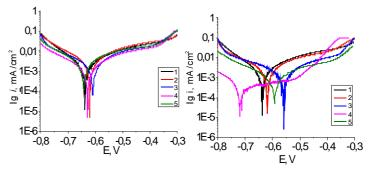
Fig. 1. The potentiodynamic polarization curves of the aluminium alloy after exposure for 24 h in 0,1% NaCl solution (1) and adding  $1 \text{ g} \cdot \Gamma^{1}(a)$  or  $2 \text{ g} \cdot \Gamma^{1}(b)$  into solution initial zeolite (2) or modified zeolite by Ca (3), Mn (4), Zn (5)
