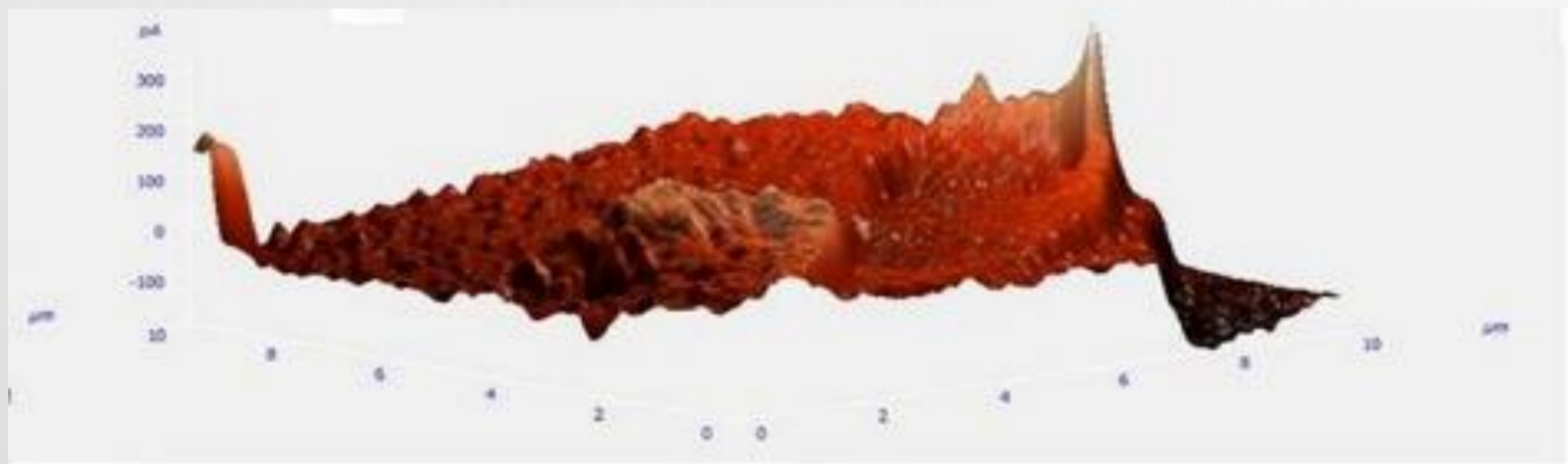
Fig. 4. PS obtained by chemical etching AFM 3D-image.
