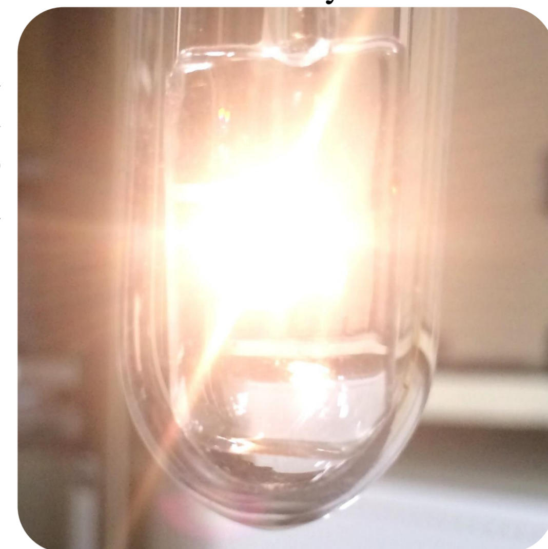
Fig. 1 The photo of LIBE under excitation at 980 nm of the (Yb_xY_{1-x})_3Al_5O_{12} nanocrystals
