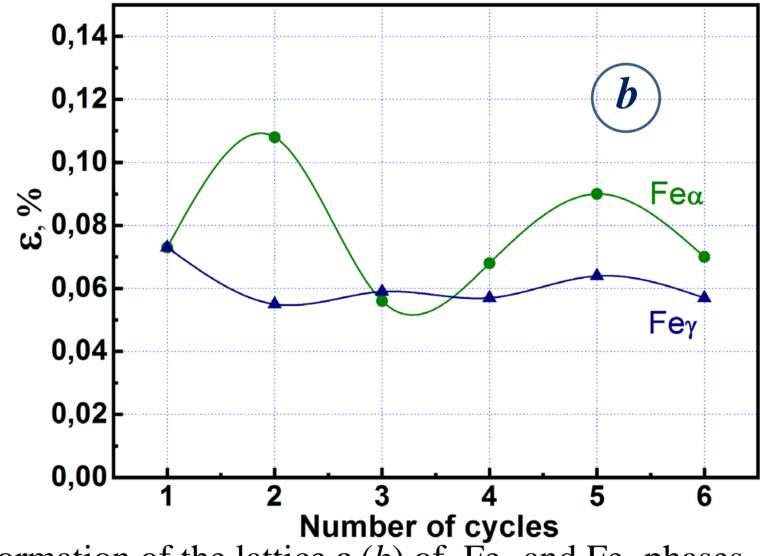
The dependences of the grain size L (a) and the related deformation of the lattice  $\varepsilon$  (b) of  $\overline{Fe}_a$  and  $\overline{Fe}_b$  phases obtained in NCS layer of  $65\Gamma$  steel from number of cycles of MPT
