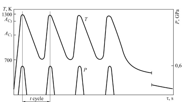
The scheme of cyclic change temperature T and pressure P in the FC zone during MPT
