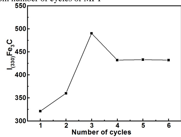
The dependence of the volume fraction of austenite phase in The dependence of the integral intensity I of Fe<sub>3</sub>C peak (330) on X-Ray the surface NCS obtained on  $65\Gamma$  steel from number of cycles of MPT diffraction patterns obtained on  $65\Gamma$  steel from number of cycles MPT
