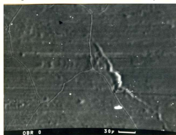
Fig.3. Surface of a crystallization-resistant nanocomposite film. Increase -500.
