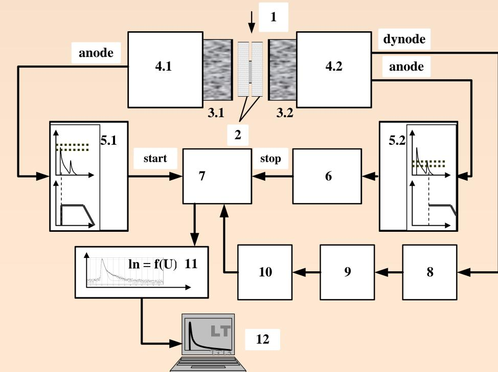
**Block-scheme of conventional sample**source "sandwich" arrangement for PAL measurements using the ORTEC apparatus:
