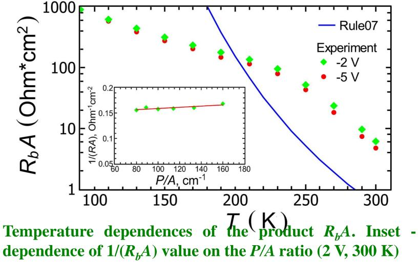
barrier layer. In this case, information on the bulk component of the current can be obtained, even if the dark current is limited by surface leakage. It can be seen that with the exception of surface leakage for this sample with a composition close to the optimal in the barrier layer (x = 0.67), diffusion-limited characteristics can be obtained.
