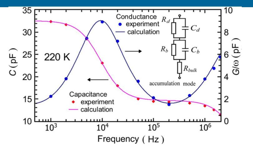
**Frequency dependences of the capacitance and normalized** conductance of the nBn structure
