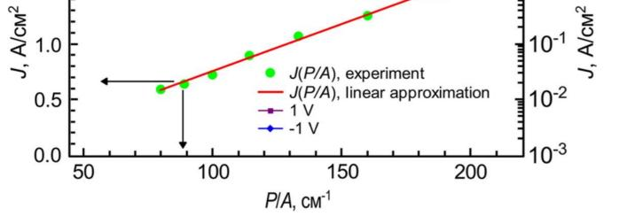
**Dependence** of the dark current density on temperature and on the ratio of the structure mesa perimeter to area (-2 V, 300 K)
