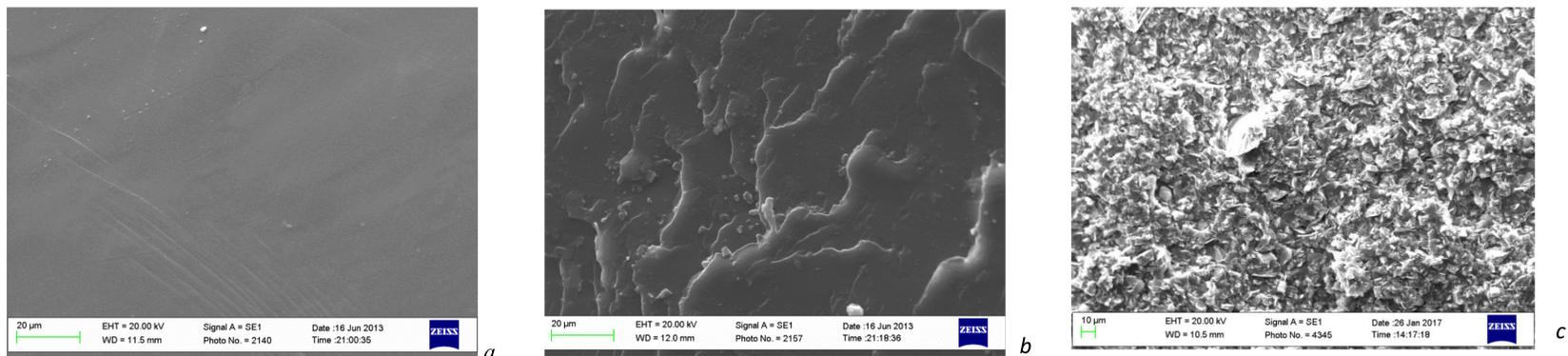
Fig. 1. Transformation of the structure of an epoxy polymer (a), with the introduction of polysiloxane particles into it (b), followed by the addition of molybdenum disulfide (c)
