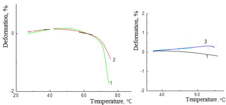
Fig. 2. TMA curves below the glass transition temperature of an epoxy polymer (1), with the introduction of polysiloxane particles into it (2), followed by the addition of molybdenum disulfide (3)
