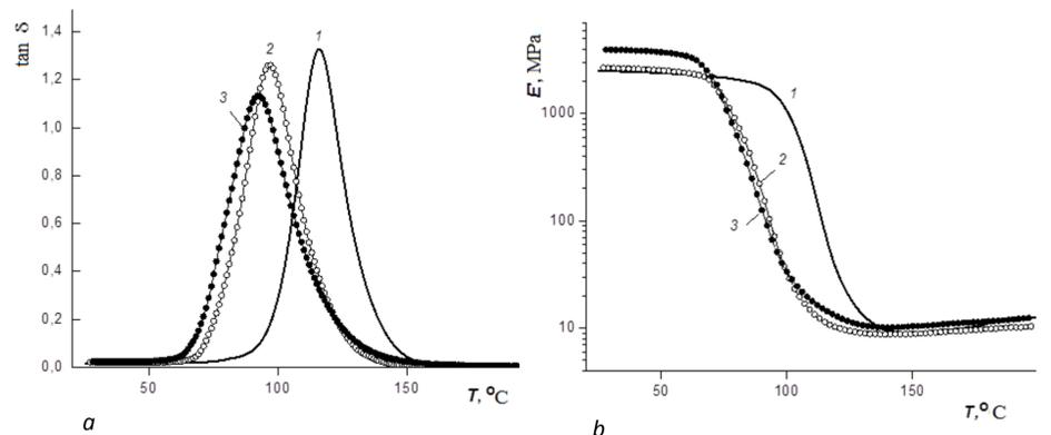
Fig. 3. Temperature dependences of the tangent of the angle of mechanical losses  $\tan \delta$  (a) and the dynamic modulus of elasticity  $E'$  (b) of an epoxy polymer (1), with the introduction of polysiloxane particles into it (2), followed by the addition of molybdenum disulfide (3)
