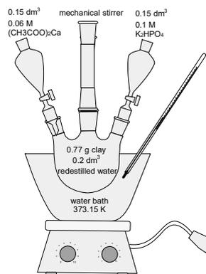
Fig.1 Synthesis of nanocomposite HA/white-blue clay
