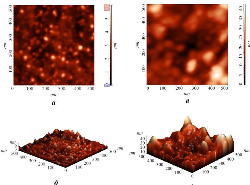
**Fig. 1.** Image of the surface morphology of  $Y_2O_3:Eu$  (a, б) and  $Gd_2O_3:Eu$  (в, г) thin films obtained by RF ion-plasma sputtering in an argon atmosphere at an activator concentration of 1 mol. %. Images a and в are two-dimensional, б and г are three-dimensional.
