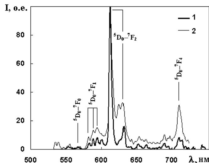
**Fig. 2.** CL spectra of (1)  $Y_2O_3:Eu$  and (2)  $Gd_2O_3:Eu$  thin films at an activator concentration of 1 mol.%. Parameters of electron irradiation pulses: electron beam current density  $j=5 \times 10^{-2} A/m^2$ ; pulse duration  $5 \times 10^{-4} s$ ; pause between pulses 0.1 s; the energy of exciting electrons is 3 keV.
