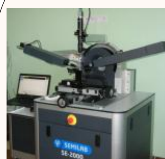
SE-2000 SEMILAB (rotating compensator) \lambda = 250-2100 nm
