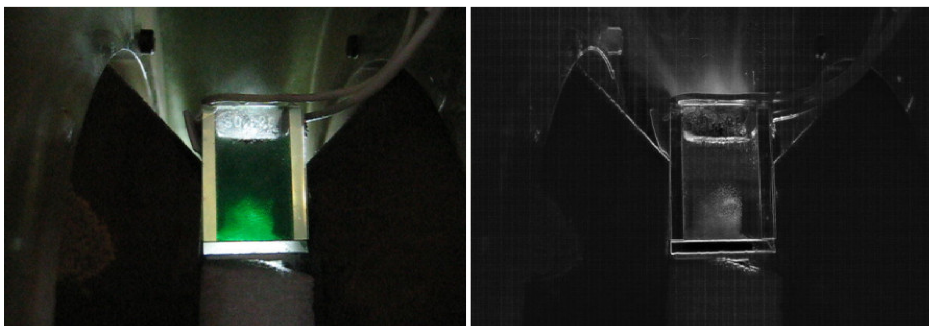
Fig. 1. Cuvette with an electrolyte in a magnetic field and the difference image obtained by processing the minima and maxima of the intensity of the sequence of 2048 frames.
