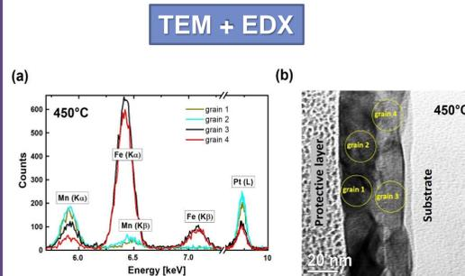
Figure 7. (a) EDX spectra and (b) corresponding cross-section TEM image of a 450°C post-annealed sample. EDX spectra were taken at specific locations of the TEM lamella as marked in (b)
