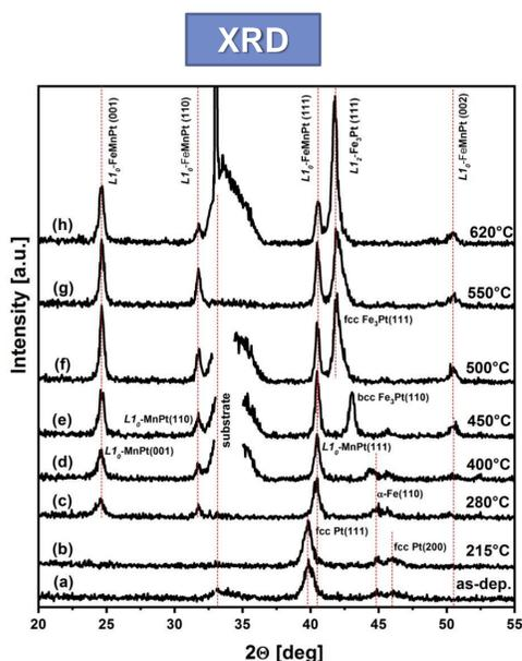
Figure 3. (a-h) XRD ( $\theta$ - $2\theta$ ) scans of Pt(15 nm)/Mn(7.5 nm)/Fe(15 nm) films after deposition and post-annealing at different temperatures.
