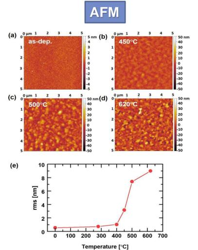
Figure 6. AFM images of the (a) as-deposited and (b-d) annealed Pt/Mn/Fe film samples and (e) temperature dependence of rms roughness.
