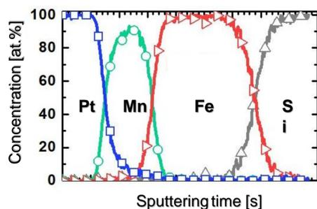
Figure 2. SNMS composition-depth profile of the as-deposited Pt/Mn/Fe film sample.
