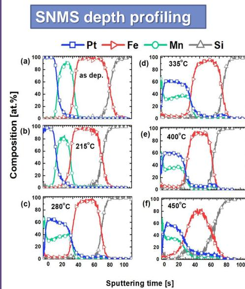
Figure 5. (a-h) SNMS composition-depth profiles of Pt/Mn/Fe films after deposition and post-annealing at different temperatures.
