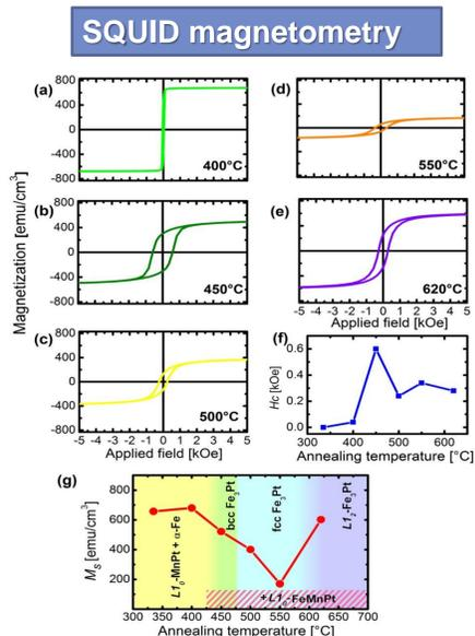
Figure 4. (a-e) In-plane M-H hysteresis loops of Pt/Mn/Fe films after deposition and post-annealing at different temperatures. (f) Coercivity and (g) saturation magnetization at room temperature as function of annealing temperature.
