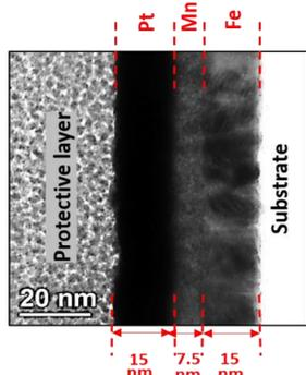
Figure 1. Cross-section TEM image of the as-deposited Pt/Mn/Fe film sample.
