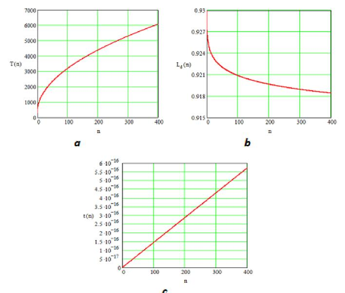
Fig. 2. Time dependence of temperature (graph a) and optical loss (graph b) (reflection only). The graph (c) is intended to translate the integer parameter  $n$  into real time (s). Here we also used the parameters for silver and the radiation flux  $7 \cdot 10^{15}$  W/m<sup>2</sup>, but for a pulse duration  $\sim 140$  fs, which is often used in real experiments.
