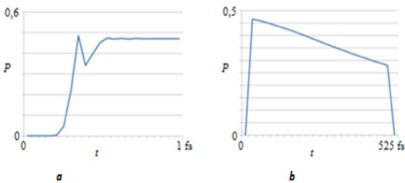
Fig. 1. Dependence of dimensionless pressure on time on the pulse axis at its maximum femtosecond duration of 500 fs at a radiation flux ( $7 \cdot 10^{15}$  W/m<sup>2</sup>): (a) the initial stage of the process  $t \leq 1$  fs; (b) the whole process  $t \leq 525$  fs
