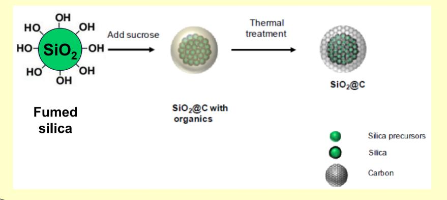
No ESR spectra were observed in  $SiO_2$ :C nanocomposites before thermal annealing. The spin concentration of the single ESR line increases with the sucrose concentration, while the thermal annealing from 300°C to 400°C quadruple the spin concentration.
