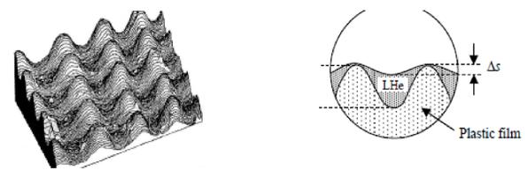
A inhomogeneities forming lattice of a wavelike micro-protrusions by step of 5x5  $\mu\text{m}$  were on film (upper peactures). Composite substrate placed on Si-plate of 0.2 mm thick at a height of 4 mm above massive helium.
