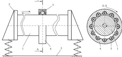
Fig. 2. Scheme of VCH of external cylindrical surfaces: 1 - sample; 2 - bracket; 3 - the general platform; 4 - tool; 5 - balls
