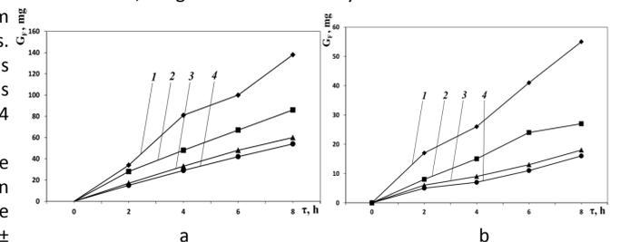
Fig. 5. Wearing kinetics for friction pairs made of 40Kh - ShKh15 steels after technological processing methods (a - ring; b - insert) under a load of 2 MPa in an oil-abrasive environment: 1 - normalization; 2 - quenching with low tempering (200 °C); 3 - VCH; 4 - MPT
