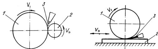
Fig. 1. MPT scheme of cylindrical (a) and flat (b) surfaces: 1 - hardening tool; 2 - work piece; 3 - technological media
