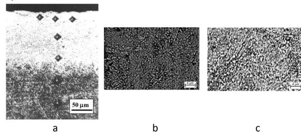
Fig. 3. The microstructure of 40Kh steel after MPT and VCH at depths: a - unetched area, b - 100  $\mu\text{m}$ , c - matrix structure of 6 mm
