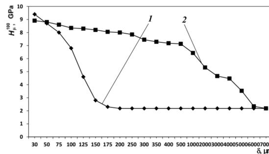
Fig. 4. Microhardness of the hardened steel layer 40Kh after various processing methods: 1 - MPT; 2 - VCH
