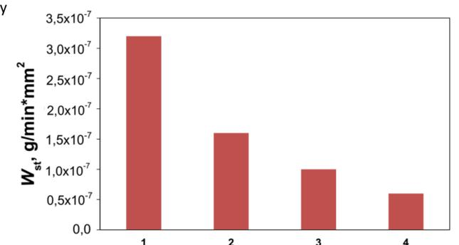
Fig. 6. The dependence of the stabilized speed of the CED on the amplitude of testing 70  $\mu\text{m}$  of samples of steel 40Kh after technological processing methods: 1 - normalization; 2 - quenching with tempering at 200 °C; 3 - VCH ( $m = 7.5$  kg,  $\tau = 28$  min); 4 - MPT
