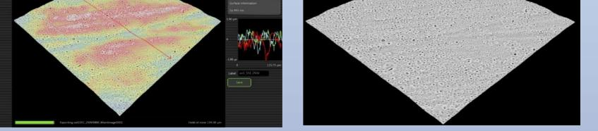
The results showed statistically significant increases (p < 0.0001) the surface roughness in the case of Sol 2 300 V (2.10±0.15) and Sol 3 300 V (2.88±0.3) samples among obtained coatings.
