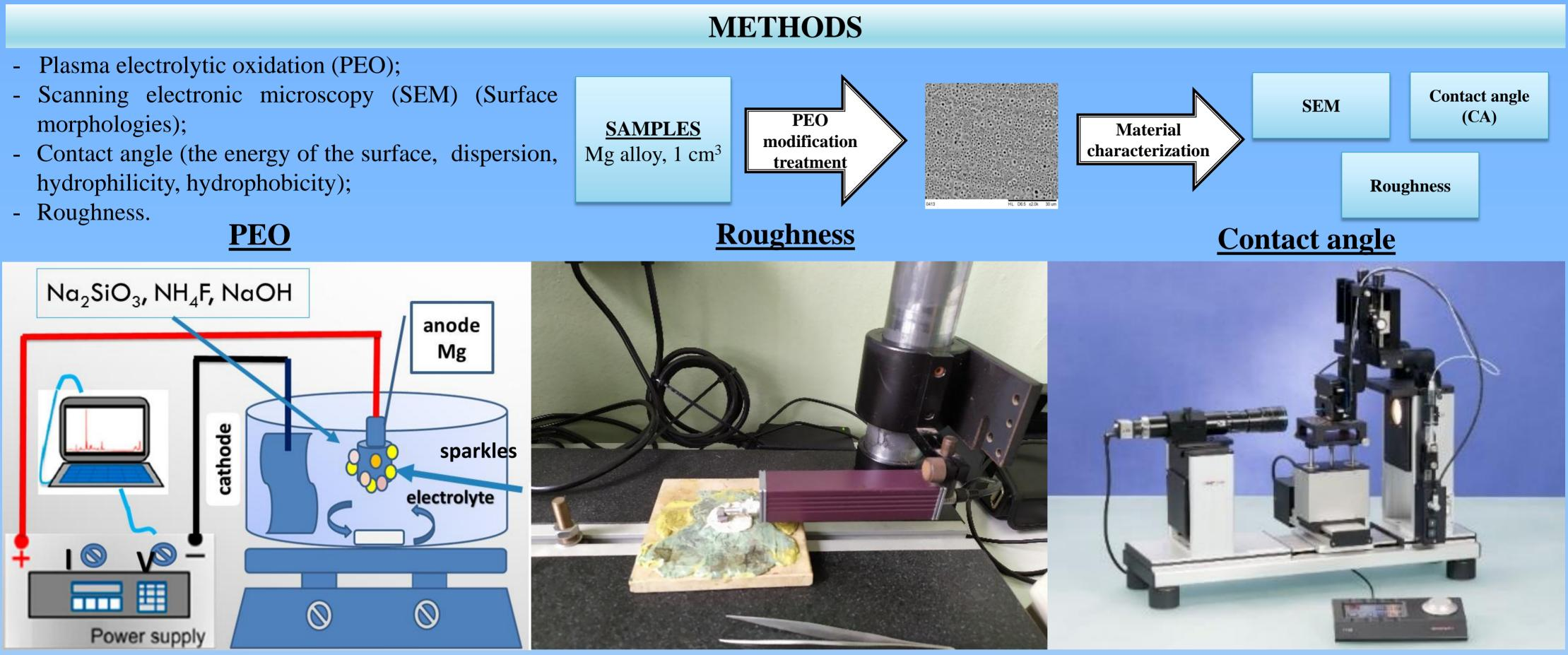
current density - 0.1 A cm<sup>-2</sup> and final voltage - 200, 250, 275 and 300 V for 10 min
