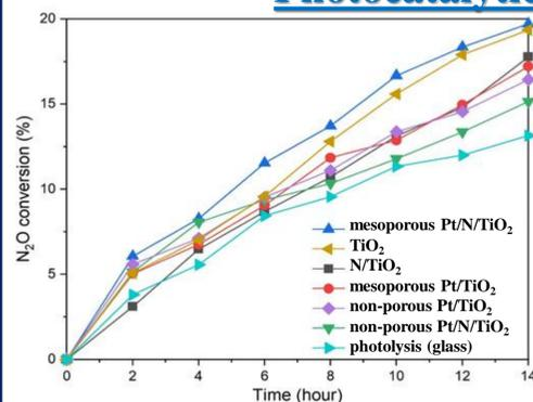
Fig. 1. Photocatalytic decomposition of N<sub>2</sub>O under UV light over TiO<sub>2</sub> and doped TiO<sub>2</sub> films
