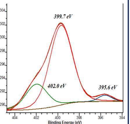
Fig. 2. XPS N1s spectrum of mesoporous Pt/N/TiO<sub>2</sub> film
