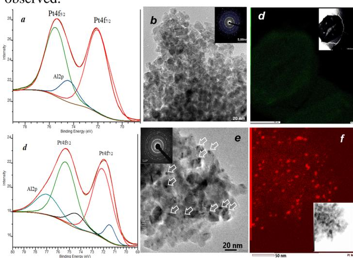
Fig. 4. XPS Pt4f spectra, TEM images and electron diffraction patterns (inserts), EDS mappings with corresponding TEM images (inserts) of non-porous (a, b, c) and mesoporous (d, e, f) Pt/TiO<sub>2</sub> films.
