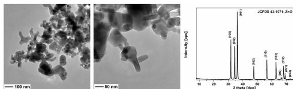
Figure 1. TEM images and XRD pattern of ZnO NPs.
