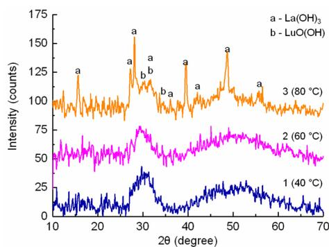
**Fig. 1** X-ray diagrams of precursor powders synthesized in ammonia solution with urea content 10 vol. % at temperature 40, 60 and 80 °C
