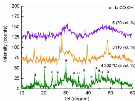
**Fig. 2** X-ray diagrams of synthesized precursors samples obtained at solution temperature of 80 °C, depending on the urea percentage
