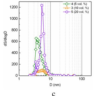
**Fig. 4** Nitrogen sorption isotherms (a) and differential size distributions of mesopores volumes (b) and surfaces (c) on synthesized precursors samples obtained at solution temperature 80 °C, depending on the urea percentage
