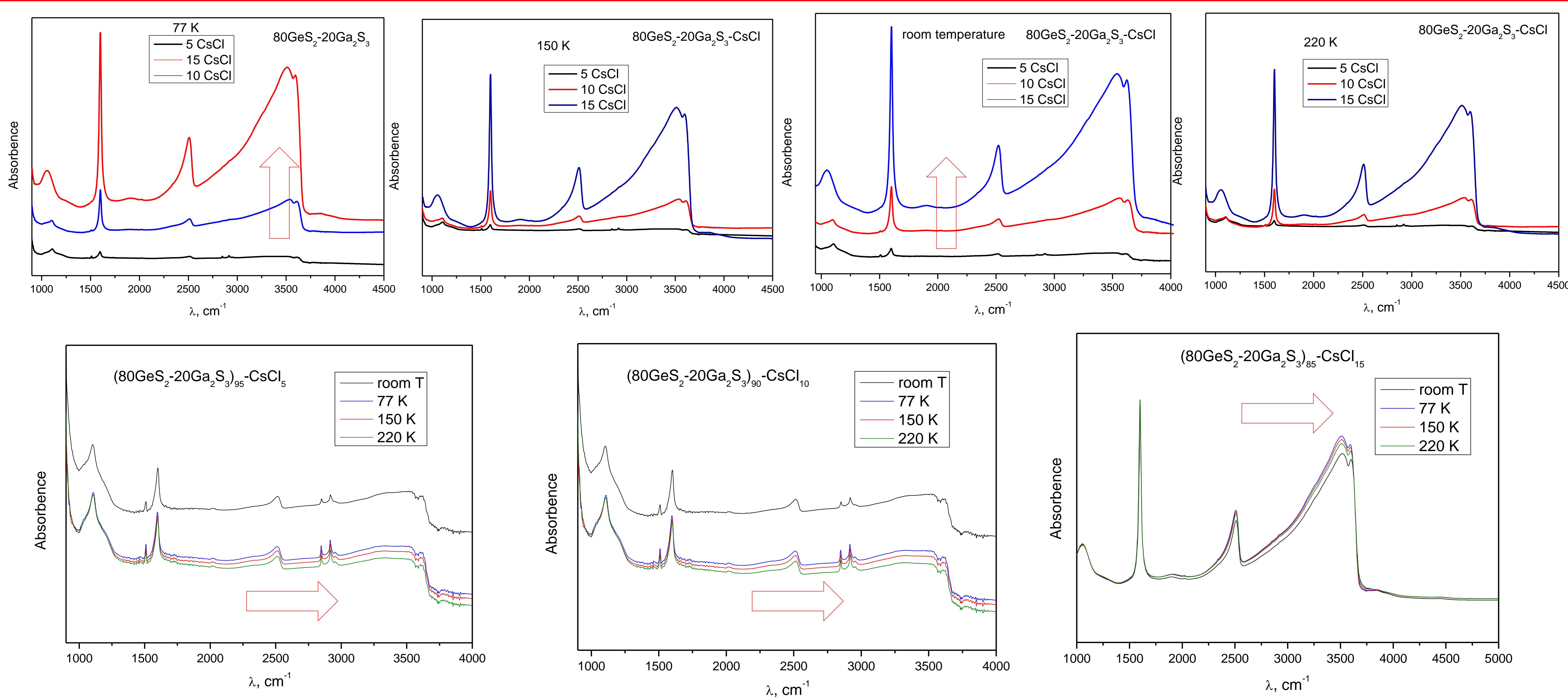
Influence of temperature on FIR spectrum of Ge-Ga-S-CsCl glasses studied by Fourier Transform Infrared (FTIR) spectroscopy measurements at 77 K, 120 K, 150 K and room temperature.
