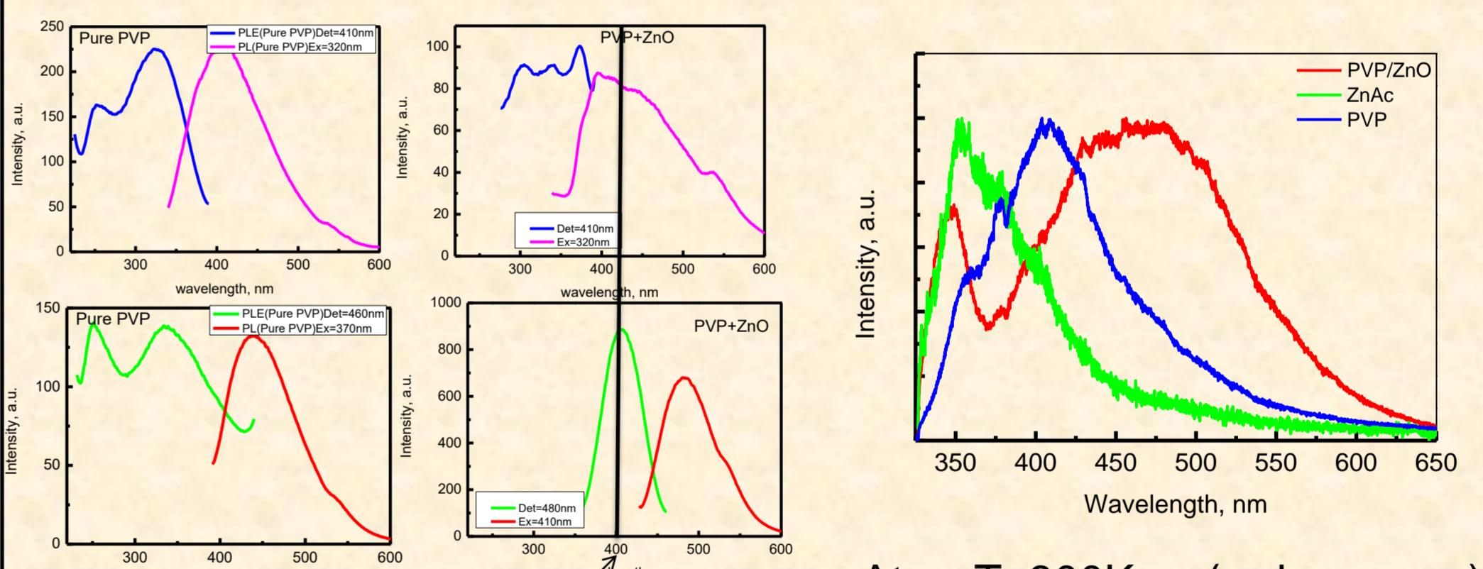
At  $T=300K$  (red curve) emission of NPs dominates in PL spectra of nanocomposite.
