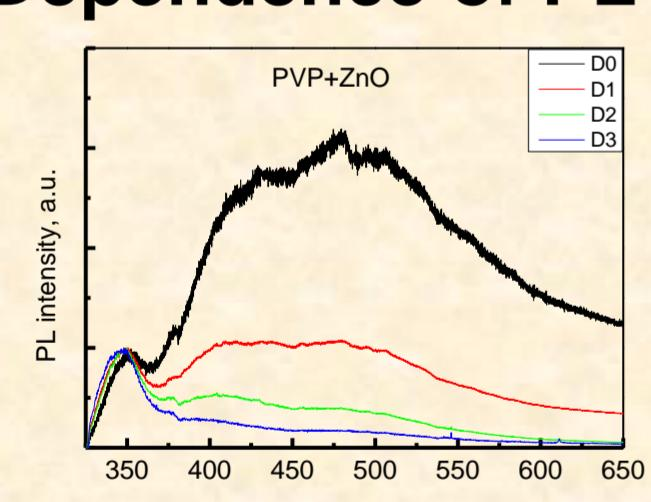
As the intensity of the exciting light increases, the contribution of nanoparticle emission to the PL spectrum of the sample increases.
