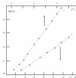
Fig. 3. I - V characteristics of the ZnO film in special coordinates (T = 293K): 1 - after several cycles of measurements in air (corresponds to curve 2 in Fig. 2), 2 - after heating to 440 K and cooling to 293 K in air (corresponds to curve 3 in Fig. 2).
