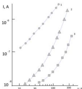
Fig.2 I - V characteristics of a ZnO film in dry air (T = 293 K): 1 - immediately after heating the film to 440 K and cooling in vacuum to 293 K, 2 - after several measurement cycles in air, 3 - after heating to 440 K and cooling to 293 K in air.
