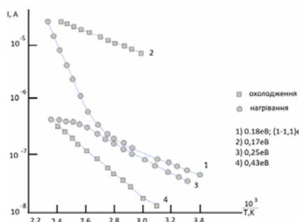
Fig. 4. Temperature dependences of the current in the ZnO film in vacuum (1,2) and in air (3,4). U = 50 V
