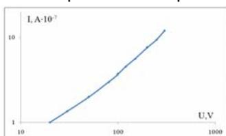
Fig.1 Volt-Current dependence of ZnO film in the open air (T=293K)
