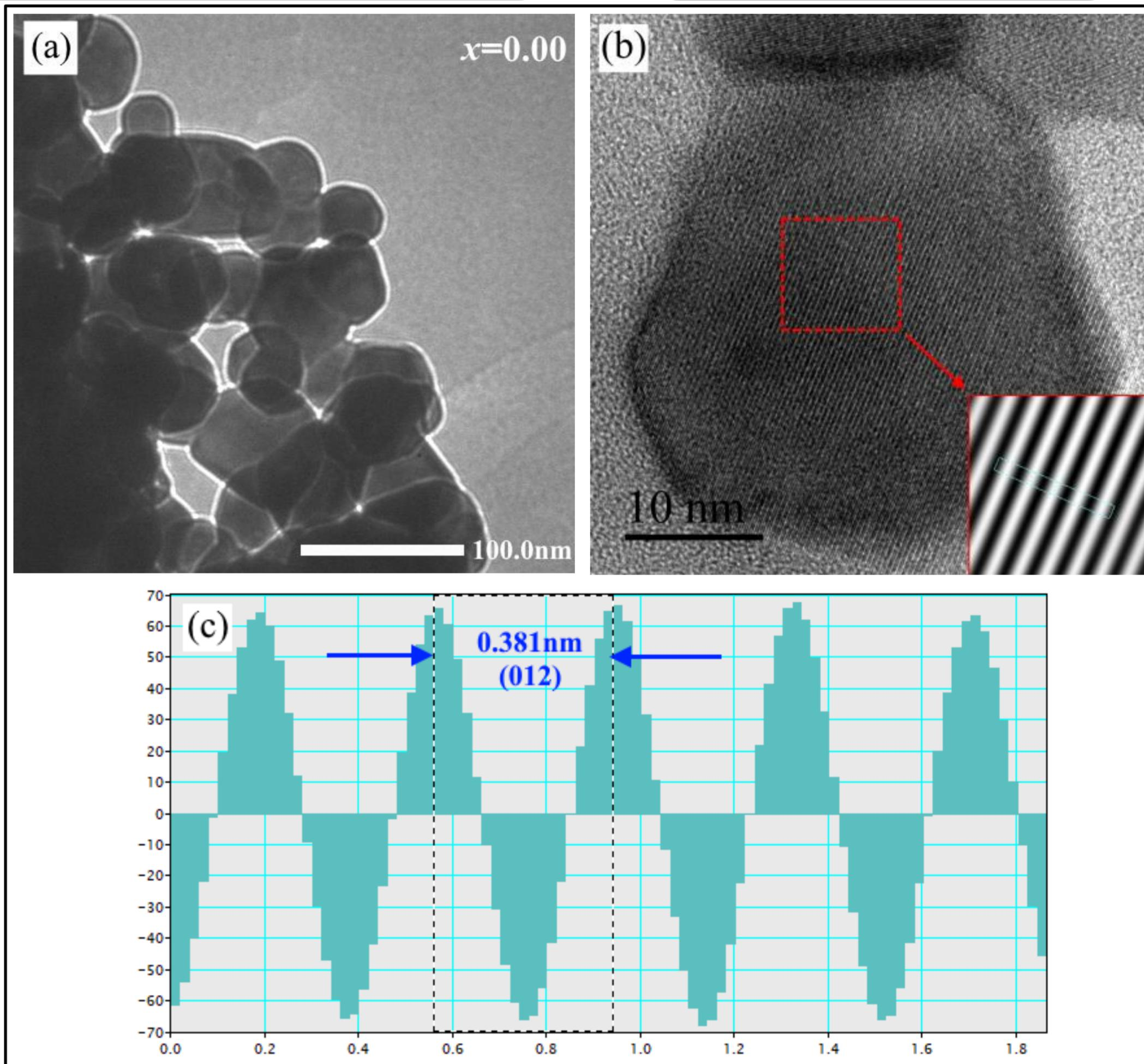
Fig. 2. TEM (a), HRTEM (the inset shows the FFT) (b), and the lattice plane intensity profile corresponding to (012) plane (c) for the  $\text{La}_{0.8}\text{Na}_{0.2}\text{MnO}_3$  nanopowder with  $t_{\text{synth}} = 900 \text{ }^{\circ}\text{C}$ .
