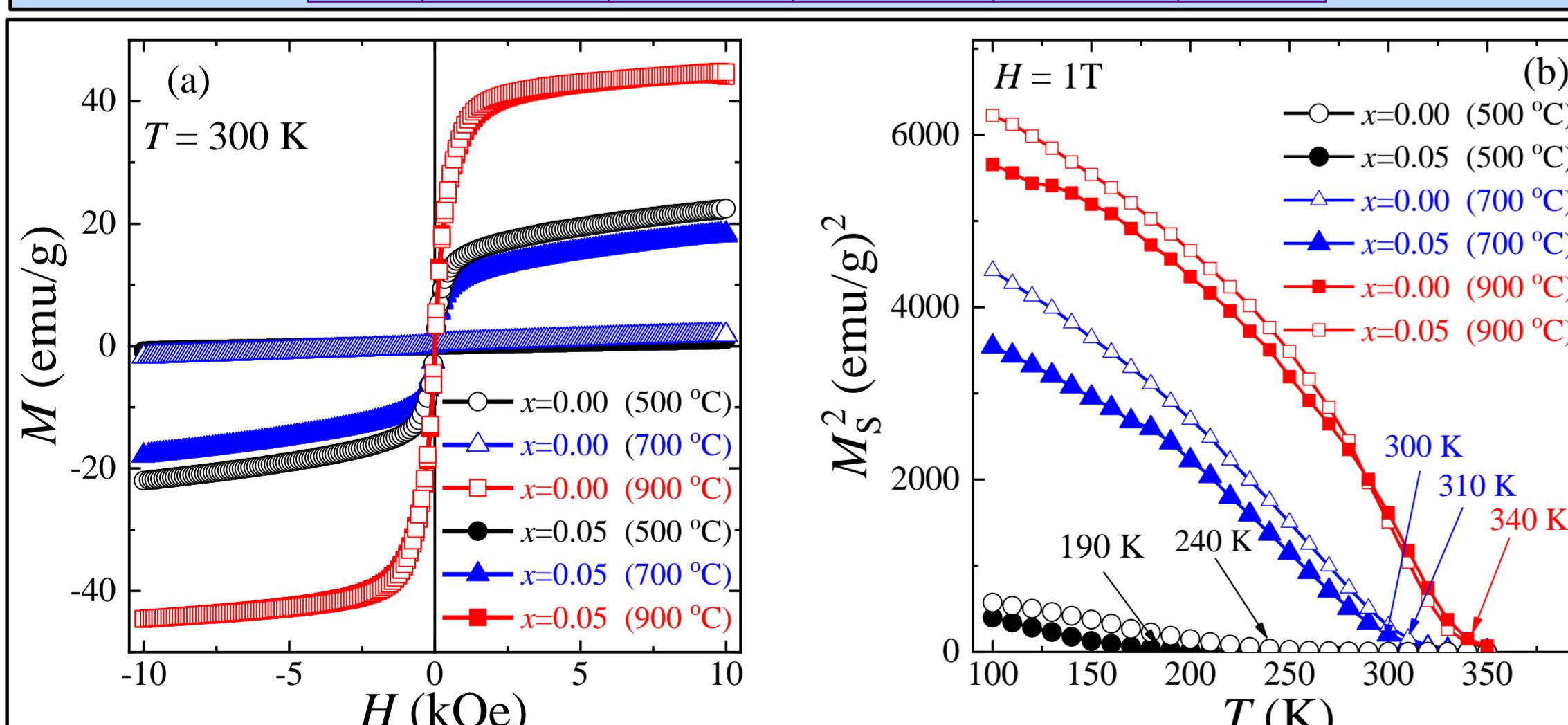
Fig. 3. Field dependences of magnetization (a) and temperature dependences of square magnetization (b) for the  $\text{La}_{0.8-x}\text{Gd}_x\text{Na}_{0.2}\text{MnO}_3$  nanopowder ( $x = 0$  and  $0.05$ ) with  $t_{\text{synth}} = 500$ ,  $700$  and  $900 \text{ }^{\circ}\text{C}$ .
