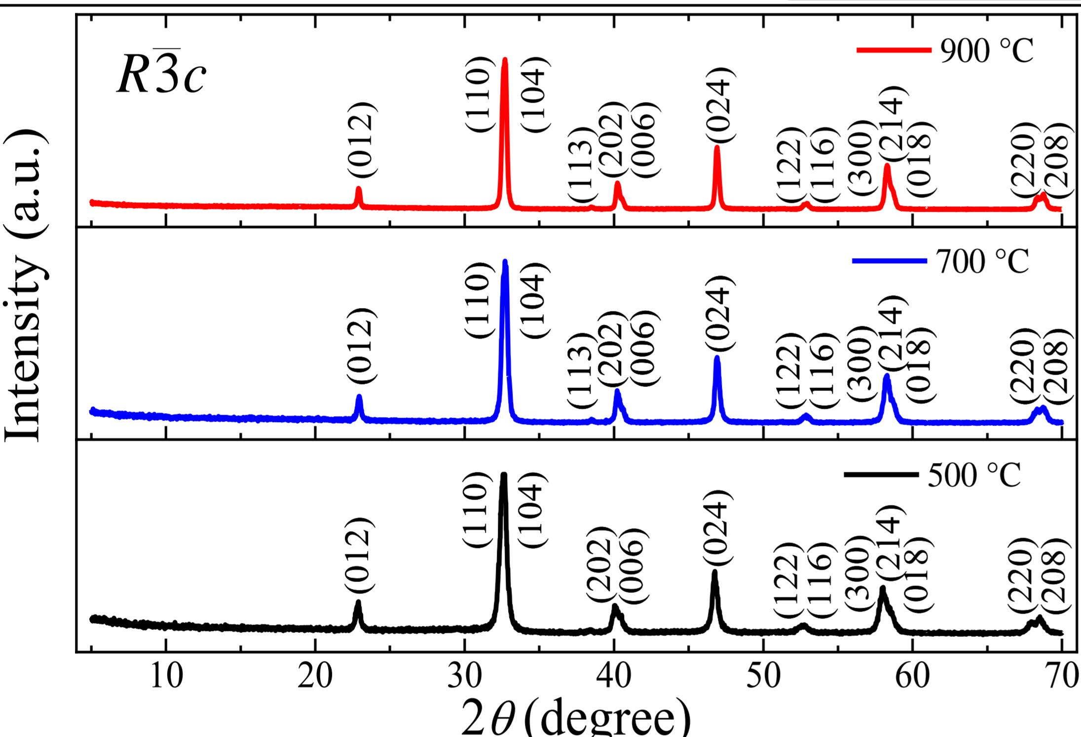
Fig. 1. X-ray patterns for the  $\text{La}_{0.8-x}\text{Gd}_x\text{Na}_{0.2}\text{MnO}_3$  nanopowder with  $x = 0$  at different additional synthesizing temperatures of  $t_{\text{synth}} = 500 \text{ }^{\circ}\text{C}$  (20 h),  $700 \text{ }^{\circ}\text{C}$  (20 h) and  $900 \text{ }^{\circ}\text{C}$  (20 h).
