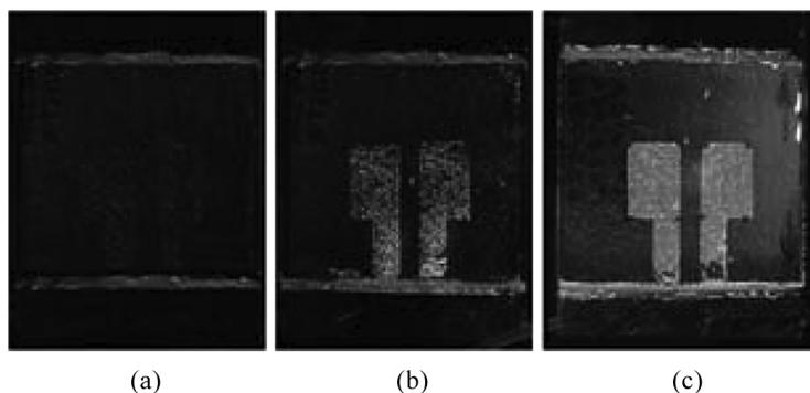
**Figure 2.** The cells filled with LC MLC6608 (a), MLC6608-CNT ( $c = 0.02$  wt.%) (b) and MLC6608-ChD-CNT ( $c = 0.02$  wt.%,  $c_{ch} = 0.1$  wt.%) (c) suspensions viewed between a pair of crossed polarizers. The rectangular areas in the middle of the cells correspond to the pixels preliminarily subjected to cycle of electric field (30 V, 1 min).
