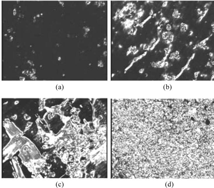
**Figure 5.** Microphotographs of two cells filled with MLC6608-CNT ( $c = 0.02$  wt.%) (a, c) and MLC6608-ChD-CNT ( $c = 0.02$  wt.%,  $c_{ch} = 0.1$  wt.%) (b, d) composition, respectively. The photos (a) and (b) show the cells before a field application, while the photos (c) and (d) show the same cells after the field application cycle (30 V, 1 min).
