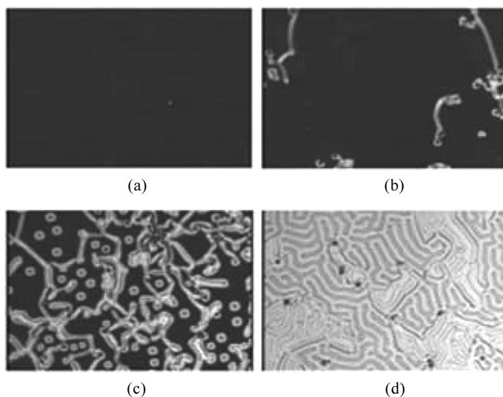
**Figure 3.** The cells filled with MLC6608-ChD compositions viewed in polarizing microscope (crossed polarizers view,  $\times 100$  magnification). The chiral dopant concentration is 0, 0.1, 0.15 and 0.2 wt.% in (a), (b), (c) and (d), respectively.
