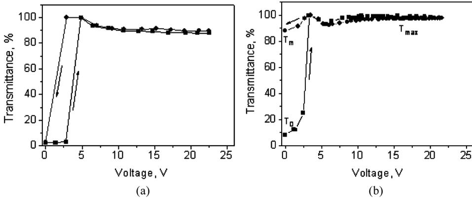
**Figure 4.** The transmittance vs. applied voltage curves for the cells filled with MLC6608-ChD ( $c_{ch} = 0.1$  wt.%) (a) and MLC6608-ChD-CNT ( $c = 0.02$  wt.%,  $c_{ch} = 0.1$  wt.%) (b) compositions. The arrows point directions of voltage ramping up and down.
