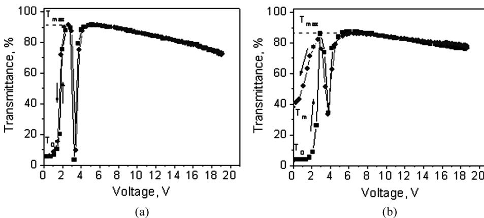
**Figure 1.** The transmittance vs. applied voltage curves for the cells filled with LC MLC6608 (a) and MLC6608-CNT suspension (b). The arrows point directions of voltage ramping up and down.
