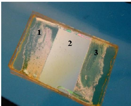
Fig. 3. Photo of symmetric cell filled with LC K15 viewed between two crossed polarizers. The cell contains P3 aligning films. The films are obliquely treated with the non-polarized UV light at the light incidence angle of  $45^\circ$ . The irradiation time is 0, 15 and 70 min in the cell sections 1, 2 and 3, respectively.
