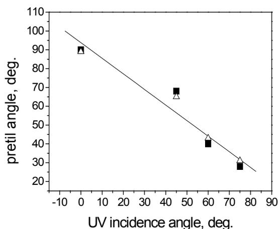
Fig. 5. The LC pretilt angle versus exposure angle plot for the P5 substrate. Squares and triangles represent results for MLC5700-000 and MLC 6610, respectively.
