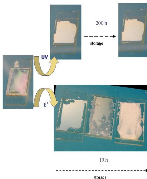
Fig. 2. The scheme demonstrating procedures of homeotropic LC alignment and its aging stability.
