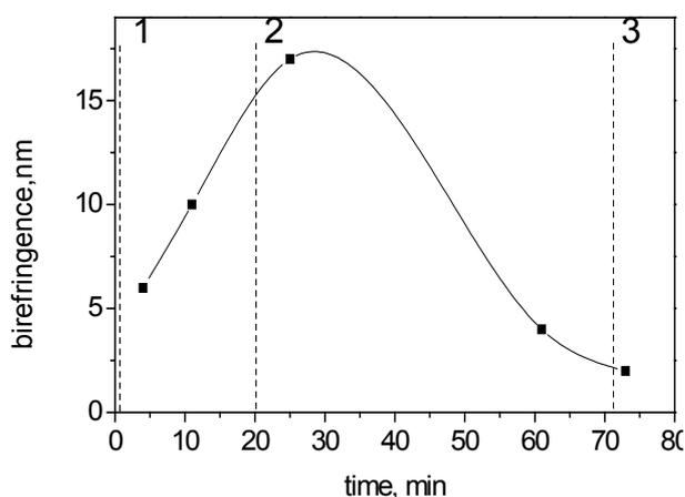
Fig. 4. The photoinduced birefringence in the film of azopolymer P3 vs irradiation time studied by ellipsometry method [4,5]. The numbers 1,2 and 3 mark irradiation doses corresponding to sections 1, 2 and 3 in Fig. 3.
