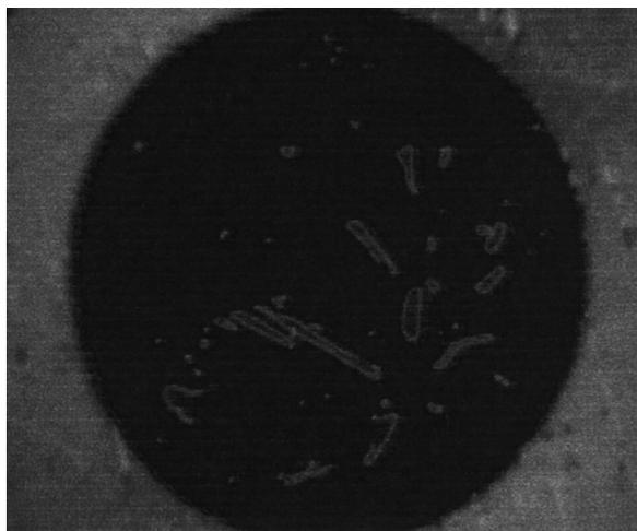
Fig. 1. A photograph of the cell in crossed polarizers. Black square in the middle part of the cell corresponds to the irradiated area.
